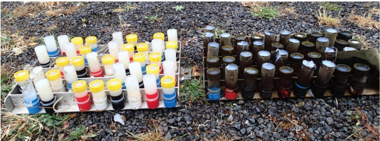
Figure 2. 15. Nutrient diffusers after 21 days of incubation, the diffusers on the left were incubated in a stream surrounded by native forest (Wairoa Tributary) and the diffusers on the right were from an urban stream (Pakuranga creek), both were removed on the same day within an hour of one another, substrates (sponge and glass) were removed for analysis.
